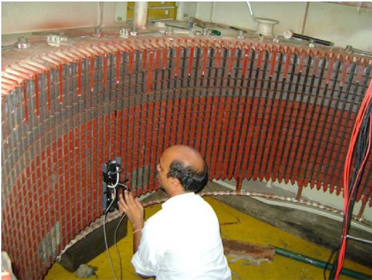
I. ELCID test performed after partial restacking of core
