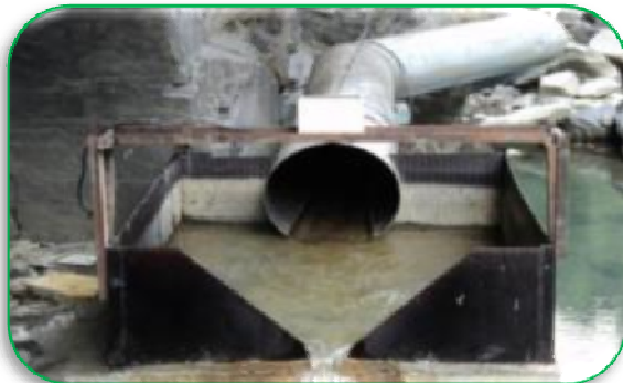
V-notch with online monitoring instrument
