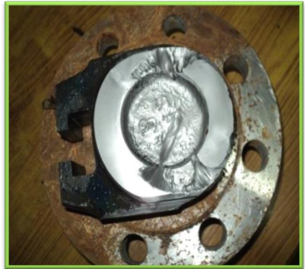
Damaged Flange with Buckler
