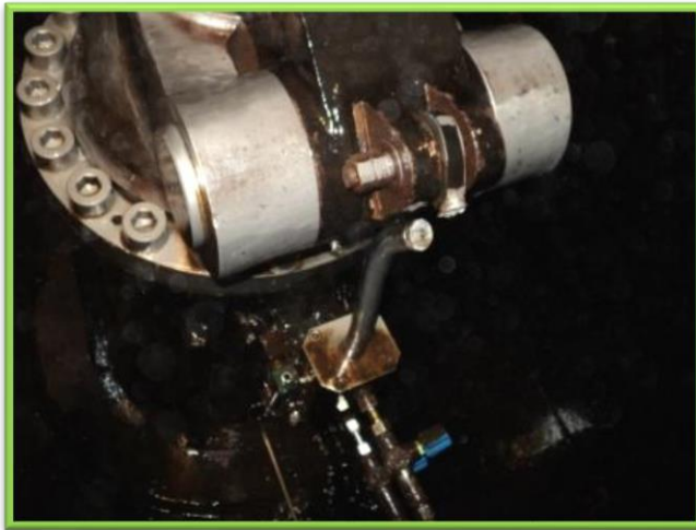
Damaged Deflector Servomotor shaft
