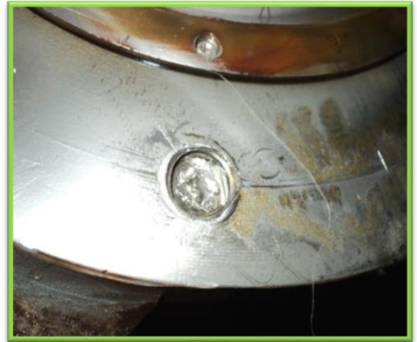
Damaged Flange with Buckler
