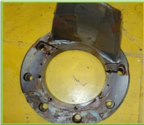
Damaged Flange with Buckler
