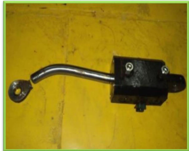
Damaged Deflector Servomotor shaft
