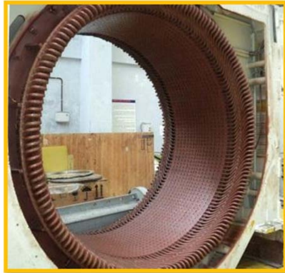
Photograph of the stator winding after restoration of wedges
