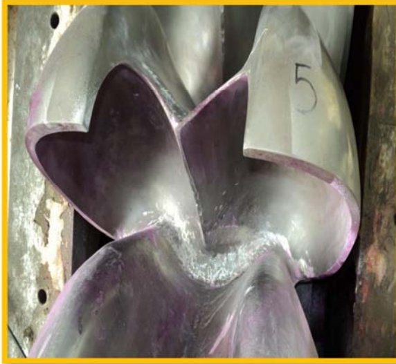
Repair work on the runner of Unit-II
