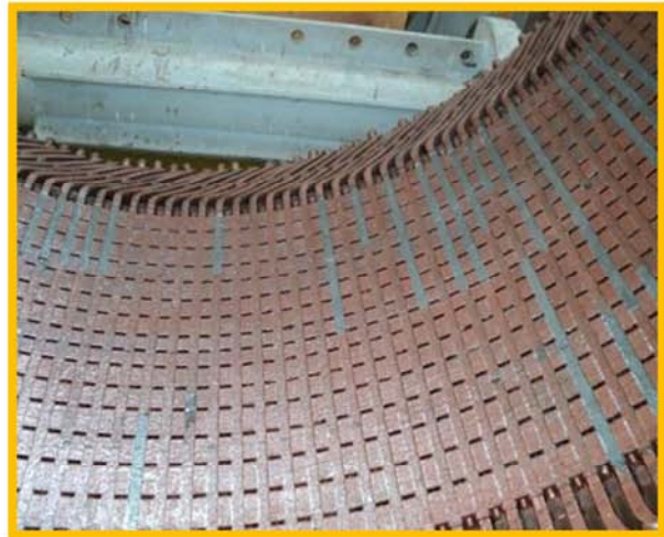
Photograph of the stator winding with misplaced wedges
