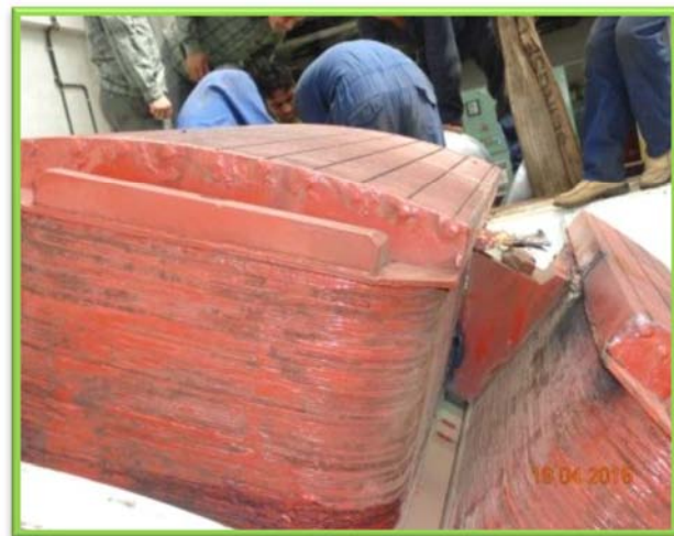
The photograph on the right shows fault at the connecting terminals and the photograph on the left shows fault in the winding inter turn area.
