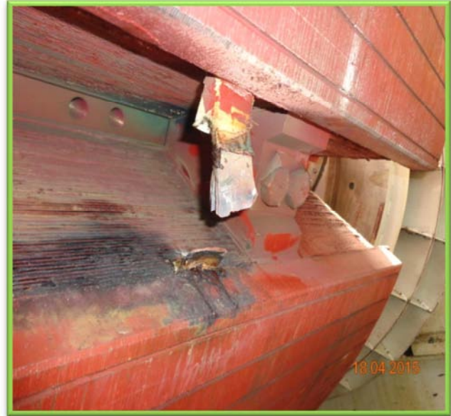
The photograph on the right shows fault at the connecting terminals and the photograph on the left shows fault in the winding inter turn area.
